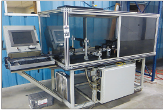
◀ WITNESS Visual Inspection System, Series 150: Sorts for Overall Length, Presence of I.D. & O.D. Threads, Damage to Parts. (7) Cameras (all upgradable), PC Touch Screen
