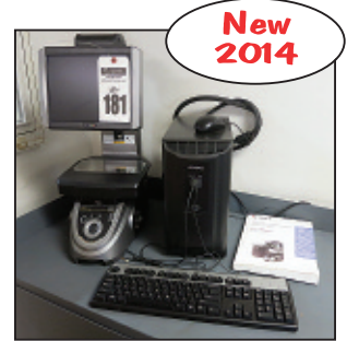
◀ WITNESS Visual Inspection System, Series 150: Sorts for Overall Length, Presence of I.D. & O.D. Threads, Damage to Parts. (7) Cameras (all upgradable), PC Touch Screen
