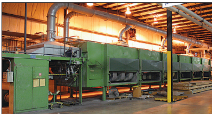
BABCOCK Saturator Line Used to Produce Melamine Impregnated Papers, Top Coated Foil or Kraft & Decorated Papers for High Pressure Laminates, Unwinder, 2-Stage Resin Bath, Immersion Baths & Top Coat, 90 - 120 FPM Melamine Paper, (3) Oven Zones, Pizzolatto A32 Rotary Knife Shear, 20' Auto Stacker
