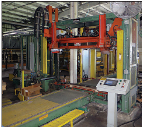
SAMUEL SLP-25 Compression Strapping System 25,000 lb. Down Force, VK30 Heat Seal Head
