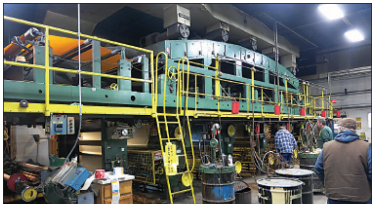
(1) Rotomack & (1) Nakajima Seiki Model GB-5 Rotogravure 5 & 6 Color/Station Printing Presses w/ Large Qty. of Printing Cylinders
