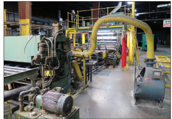
Vinyl Lamination Line 62" Wide, 1/2" - 1-1/4" Thick, 10' Long, Forklift Unload Station, Elevator Platform, Brush Cleaning, Conveyor Rolls, Pre-Heat, Black Brothers Gluer, Flash Over, Laminator, Knife Shear, Embosser, Cross Transfer Tables
