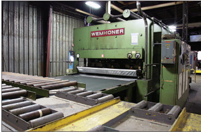
WEMHONER Short Cycle Hydraulic Laminating Press 8' x 16' Press Area - (4) 4' x 8' Sheets at Once, 60 - 80 Loads per Hour, 200°F - 250°F, Auto Board Feeder and Handling Equipment, New 1981
